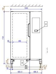
ΕI 452 R0 **DUTLET EXT Ø22mm** INLET EXT Ø12mm
